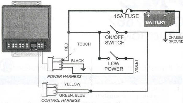
Touch YELLOW to the terminal of the RED wire to select flash pattern. Connect YELLOW to GROUND to ensure that flash pattern will never change.
