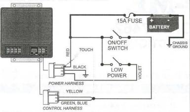
Touch YELLOW to the terminal of the RED wire to select flash pattern. Connect YELLOW to GROUND to ensure that flash pattern will never change.
