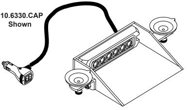
To change flash pattern, press the momentary switch (Located on the plug adaptor). Each time the momentary switch is pressed, the flash pattern will change. Less than 1 second for next pattern. About 3-5 seconds for steady burn. More than 5 seconds to turn off.
