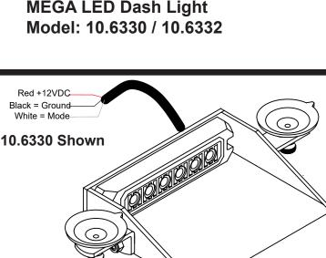
To change flash pattern, momentarily apply +12 VDC to White wire. Each time +12 VDC momentarily applied to the White wire, the flash pattern will change. Less than 1 second for next pattern. About 3-5 seconds for steady burn. More than 5 seconds to turn off.
