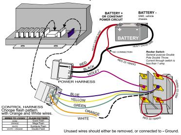
**DIAGRAM (3):** Selective switching of strobe head pairs. Low Power selection. Choose flash pattern from chart.
